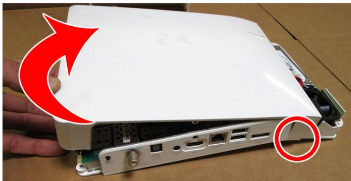
Figure 8b – Removing large lid step 2
