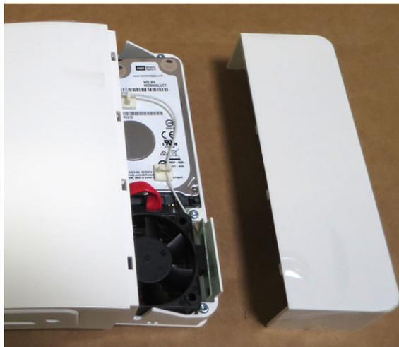
Figure 6 – Removing side lid
