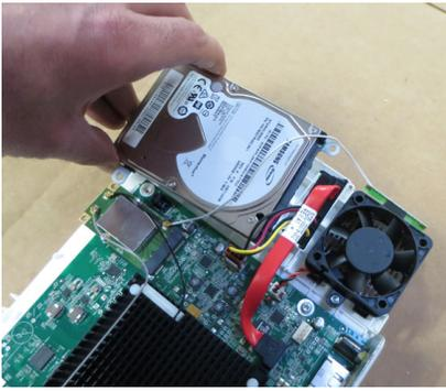
Figure 12 – Installing new hard drive
