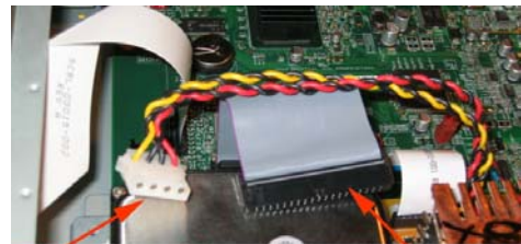
Power cable (rounded side up) IDE cable (notch up)
