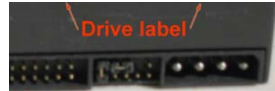
Two-jumper Maxtor Set as “Master”
