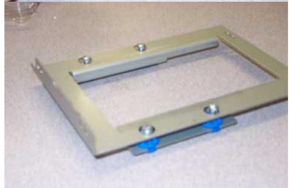
**STEP 4:** Align the bracket on the hard drive as shown. The ends of the four screws should align with the holes in your hard drive. Be sure to orient the drive and bracket as shown in the picture: The hard drive's IDE and power connections should be at the end of the bracket with the L-shaped bend.
