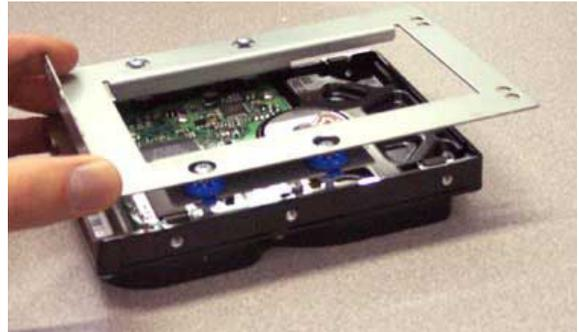
**STEP 5:** Find the two pegs in the TiVo and install the bracket next to the other bracket (if it's still in the TiVo), being sure to get the pegs through the new bracket. One peg is circled in the picture.
