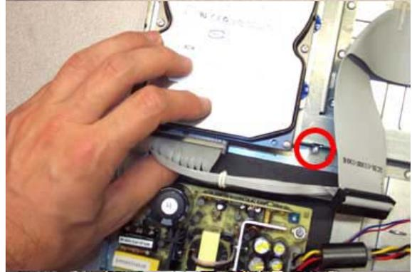
**STEP 6:** Insert a washer into the end of each of the self-tapping screw. Using the self-tapping screws and a Phillips head screwdriver, secure the bracket to the TiVo. The self-tapping screws (and washers) should be inserted into the bracket holes near the front of the TiVo. Please note that you will be cutting threads in the metal holes, so it might require a bit of force to get the screws started.
