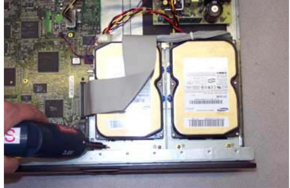
If you purchased a dual-drive kit, you should now screw in the "A" drive/bracket into the TiVo. Use the two short Torx T-10 screws that you removed in Step 4.
